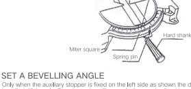
Only when the auxiliary stopper is fixed on the left side as shown the drawing, the sawblade can be bevelled 45 ° angle. To adjust a bevelling angle, loosen the fixed handle ,then incline the sawblade to the left until the indicator reaches the desired angle on the miter square, tighten the fixed handle ∕liter square
